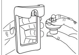
5. Align Hook opening with notches in the handle. Push up on seat cup so the stem rises.
