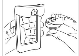
7. Hand tighten upper assembly to body by twisting bonnet clockwise.
